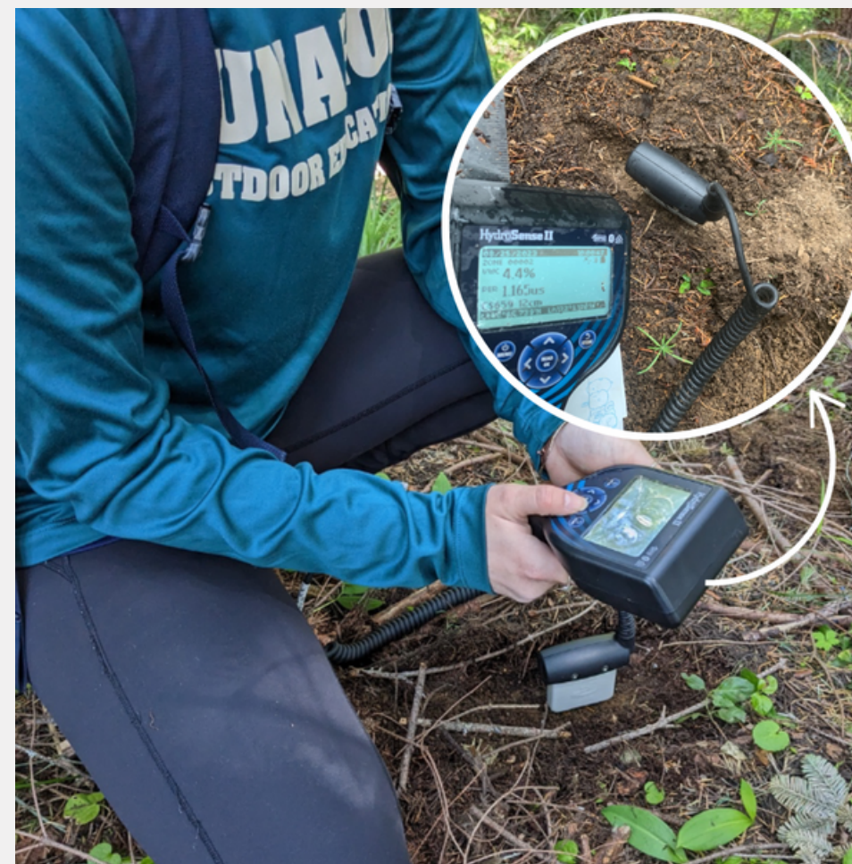
Figure 2: Niki (NNRG intern) taking soil moisture measurements using a soil moisture probe. The inset image shows the soil horizons and the probe's console. The probe reads soil moisture in volumetric water content (VWC%) and how long the reading took in microseconds (μs).
